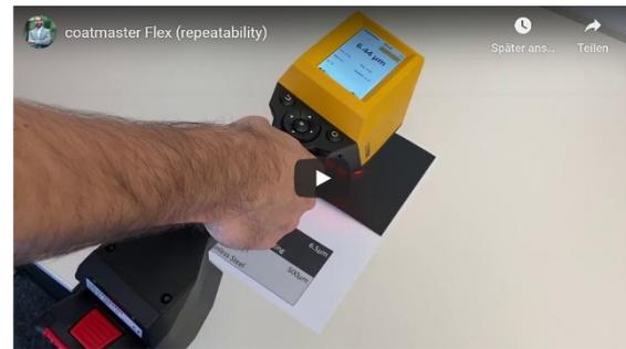
2 Video: coatmaster Flex measures the coating thickness of an e-coat on sheet metal accurately and precisely (test of repeatability)
