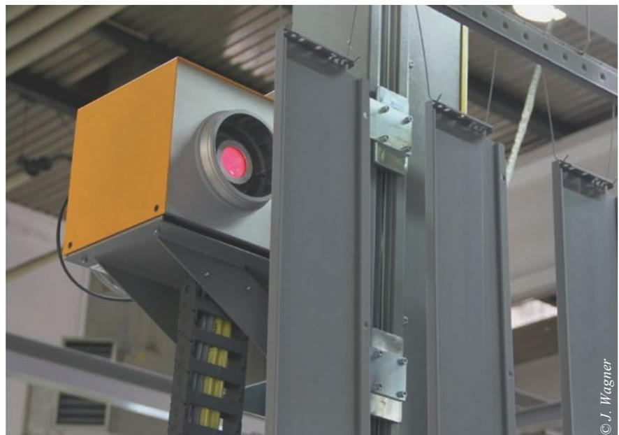
The coating thickness is measured continuously before curing from a distance of between 5 and 50 cm. Measurements can also be made on moving and tilted parts.
